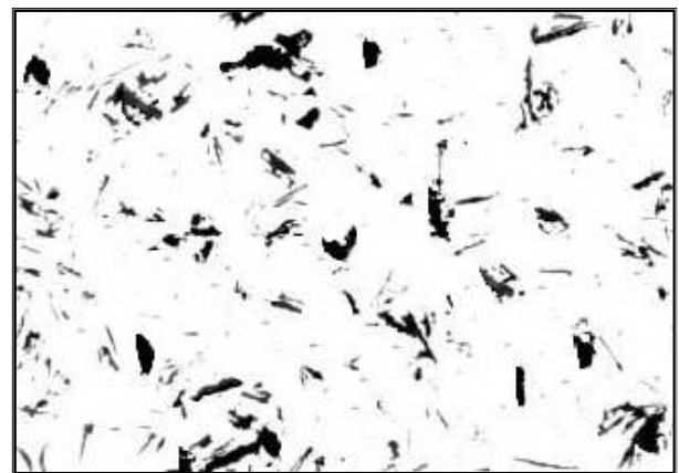
Fig. 4. Microstructure of AlMg10/ 15% C_{gr} composite of AlMg10 matrix alloy composite reinforced with 15% of graphite particles
