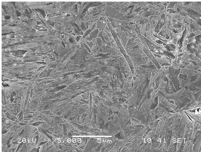
Fig. 8. Microstructure of the sample SA 860 Q (Soft annealing / quenching from 860°C), 679 HV10
