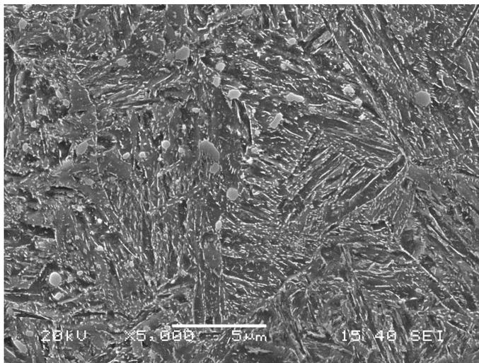
Fig. 10. Microstructure of the sample SA 840 QT (Soft annealing / quenching from 840°C / tempering), 424 HV10
