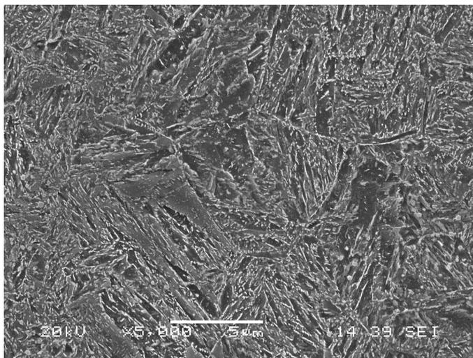
Fig. 9. Microstructure of the sample ASR 840 QT (ASR / quenching from 840°C / tempering), 446 HV10
