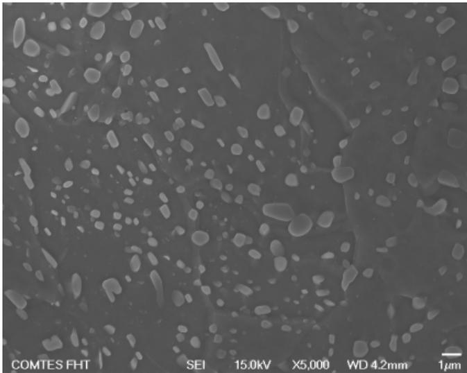
Fig. 4. Microstructure after soft annealing (SA), 179 HV10
