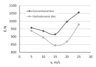
Fig. 7. The effect of drawing speed on the drawing force magnitude for wires drawn in conventional and hydrodynamic dies (the last draw)
