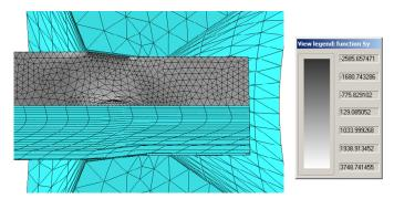
Fig. 2. A sample distribution of  $\sigma_y$  longitudinal stress in finished  $\phi 1.70$  mm-gauge wires drawn in hydrodynamic dies at a drawing speed of 25 m/s
