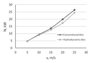
Fig. 6. Variation in drawing power (in the last draw) as a function of drawing speed for wires drawn conventionally and hydrodynamically
