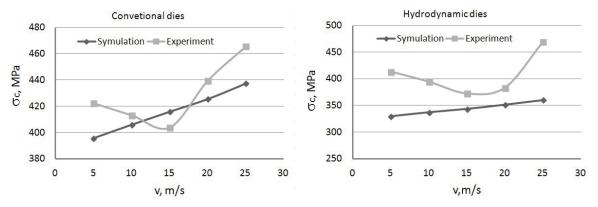
Fig. 11. Variation in drawing stress in the last draw as a function of drawing speed for wires drawn in conventional and hydrodynamic dies
