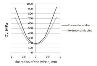
Fig. 3. The distribution of longitudinal stresses as a function of wire radius *R* for  $\phi 1.7$  mm-gauge wires drawn at speed 25 m/s in conventional and hydrodynamic dies, respectively
