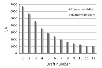
Fig. 8. Variation in the magnitude of drawing force in individual dies for wires drawn in conventional and hydrodynamic dies (at v = 25 m/s)
