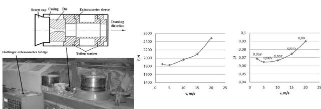
Fig. 1. The stand for the measurement of the drawing force on the Koch multi-stage drawing machine (drawing wire from the diameter of  $\phi$ 1.85 mm to  $\phi$ 1.7 mm) and the measured values of the drawing forces *F* and the friction coefficients  $\mu$  [11]
