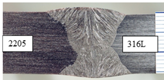
Fig. 2. Macrostructure of dissimilar 2205 – 316L welded joint
