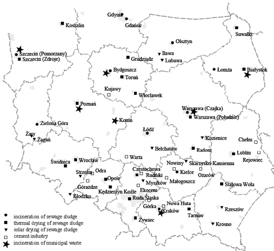
Fig. 6. Thermal utilization of sewage sludge in Poland (Bień, 2013)
