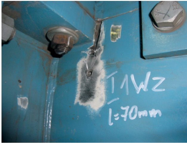
Fig. 2. Crack on the contact point between the shield and the side disc
