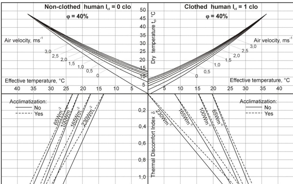
Fig. 2. The nomogram for thermal discomfort assessment, relative humidity  $\phi = 40\%$
