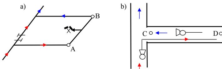
Fig. 6. Location of measuring points in: a) a longwall, b) a heading.
