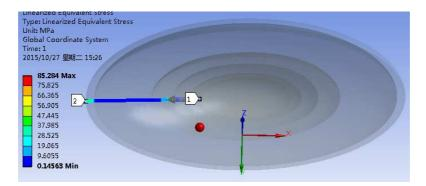
Figure 29: Radial linear stress.
