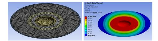
Figure 21: Grid division and temperature stress contour of ellipsoid.
