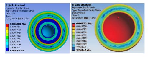
Figure 8: Equivalent elastic strain.
