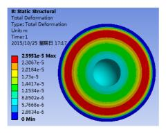
Figure 12: Total deformation contour of sphere structure.
