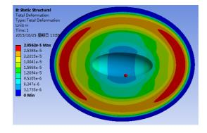
Figure 20: The total deformation contour of ellipsoid.
