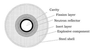
Figure 1: Schematic diagram of complicated multiplelayer components.
