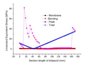
Figure 26: Four kinds of radial linear stress.
