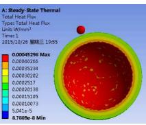
Figure 6: Heat flow density contour.
