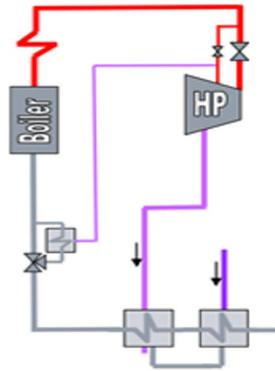
Figure 9: Top feed water heater arrangement.
