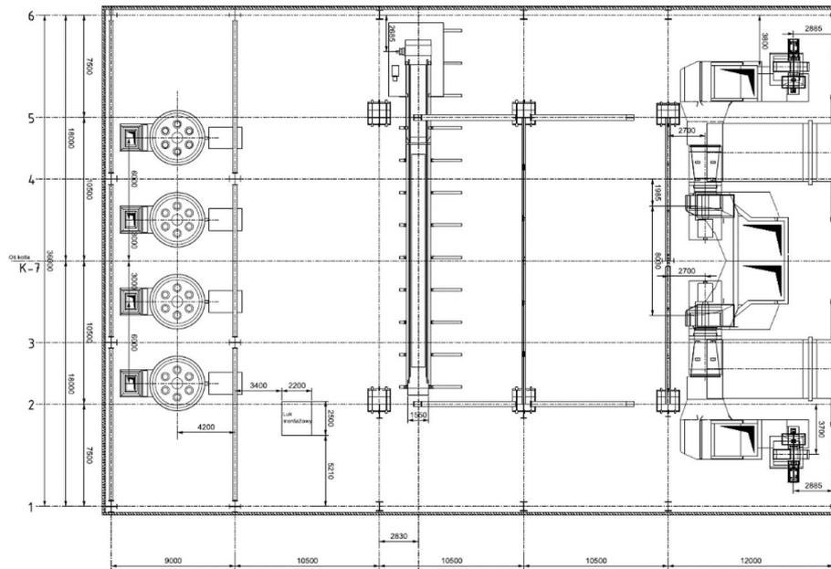
Figure 13: Typical boiler house 0.00-m elevation layout in Polish 200-MWe units.
