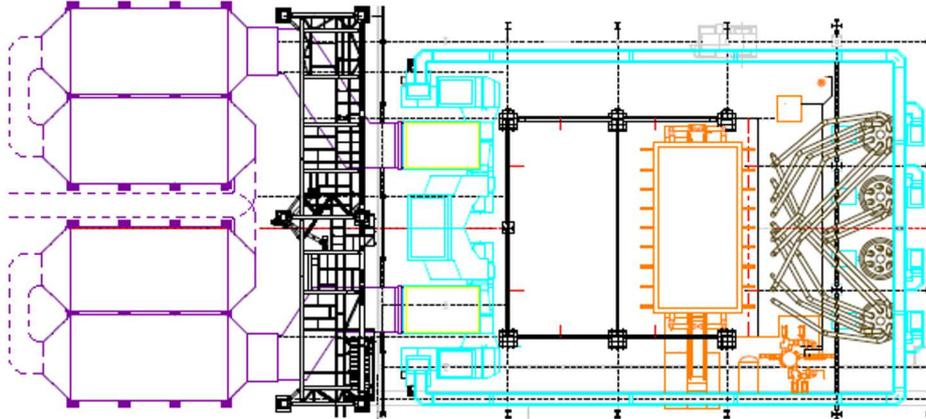
Figure 15: DuoBlock's boiler island for Koziencice.
