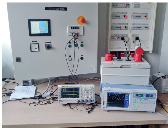
Fig. 8. Experimental setup of three-level AC-DC converter
