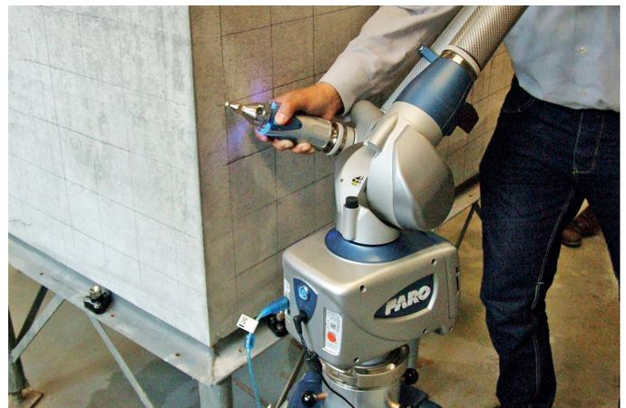
Fig. 6. Tank during measurements and visible reference points placed on a supporting steel frame
