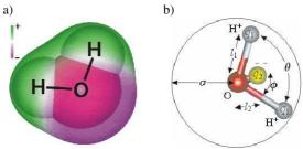
Fig. 1. Water molecule: a) the structure of a water molecule illustrating the density and distribution of electric charge.b) a schematic representation of the TIP4P molecular model geometry of a water molecule for the simulation:  $l_1=0.9572\cdot 10^{-10}$  m,  $l_2=0.15\cdot 10^{-10}$  m,  $q_1=+0.5200,\ q_2=-1.0400,\ \theta=104.52^\circ,\ \phi=52.26^\circ.$  The value of the charge is related to the value of elementary charge,  $1.60^*10^{-19}$ C, after Ref. 18
