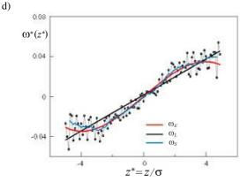
Fig. 6. Distributions of water microrotation at  $Fx^*=2.5$  in the copper (a), (c) and quartz channels (b), (d): in the narrower (a), (b) and wider ones (c), (d) with approximating curves obtained from:  $\omega_E$  – analytical solution (2),  $w_l$  – linear function. Points o denote the values from the simulation
