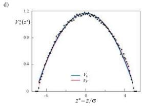
Fig. 5. Water velocity distributions at  $Fx^*=2.5$  in copper (a), (c) and quartz (b), (d) channels: in the narrower (a), (b) and the wider ones (c), (d) with approximating curves obtained from:  $V_E$  – analytical solution (1),  $V_T$  – Travis' curve. Points o denote the values from the simulation
