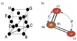
Fig. 2. Schematic representation of the geometry of molecular material models: a) elementary copper crystal after Ref. 14, b) geometry of the molecular model of a single quartz molecule;  $l_1=1.60\cdot 10^{-10}$  m,  $\theta=109.28^\circ$ ,  $q_2=+2.4$ ,  $q_1=-1.2$  after Ref. 18. The value of charge is related to the value of elementary charge,  $1.60^*10^{-19}\mathrm{C}$ , after Ref. 13
