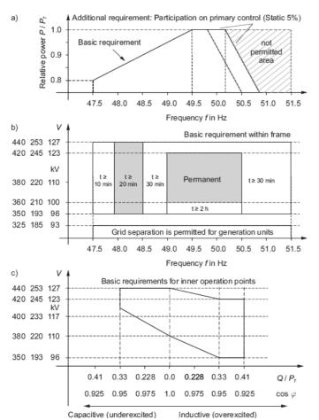
Fig. 1. Grid connection requirements for WTs in Germany after Ref. 5: a) power curve; b) supply duration; c) reactive power supply
