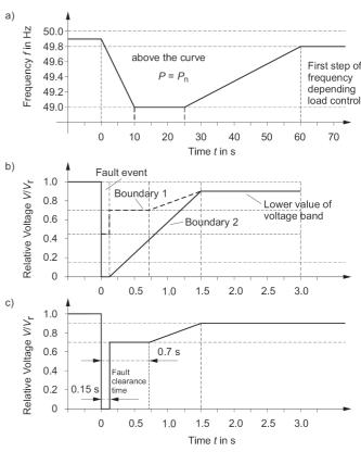
Fig. 2. German low voltage fault-ride-through guidelines for: a) low frequency; b) low-voltage after Ref. 5; c) short-circuit close to generator after Ref. 6
