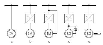
Fig. 3. Generator types: a) direct coupled induction machine; b) induction machine with full-size VSI; c) double-fed induction machine; d) electrical excited synchronous generator with VSI; e) Synchronous Generator (SG) with permanent magnet excitation
