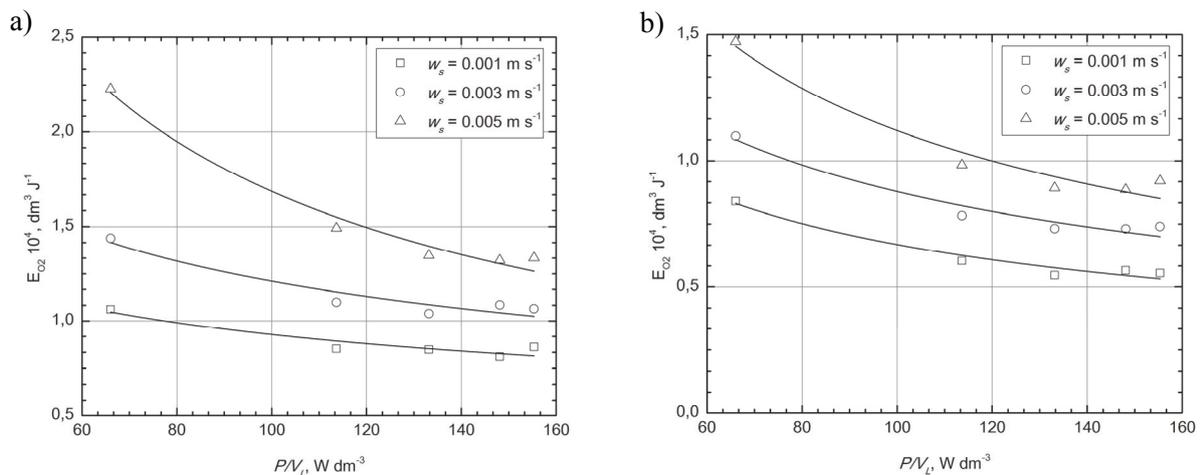
Fig. 9. The influence of specific power input on oxygen transfer efficiency
