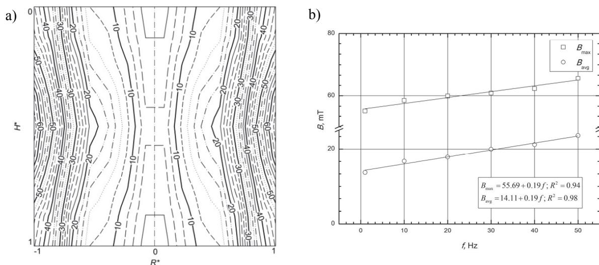
Fig. 3. A typical example of spatial distribution of the magnetic field in the cross-section of the RMF generator for  $f = 30$  Hz (a) and the graphical presentation of the relations between the maximal ( $B_{\max}$ ) and the averaged ( $B_{\text{avg}}$ ) values of magnetic induction versus the frequency of the excitation current  $f$  (b)
