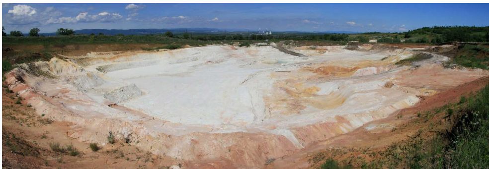
Fig. 6. Kaolin deposit Rokle in the Kadaň region is producing mostly paper-grade kaolin. Parent rock is fine to medium-grained granulite orthogneiss Phot. Jaromír Starý 2016
