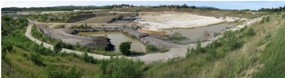
Fig. 2. Kaolin deposit Božičany-Osmosa in the Karlovy Vary region, producing all grades of kaolin (kaolin for production of porcelain and fine ceramics, for other ceramics manufacturing, and titanium-bearing). Elevation of medium-grained muscovite-biotite granite weathered in Tertiary, since Late Oligocene lignite seam is in direct kaolin overburden Phot. Jaromír Starý 2016
