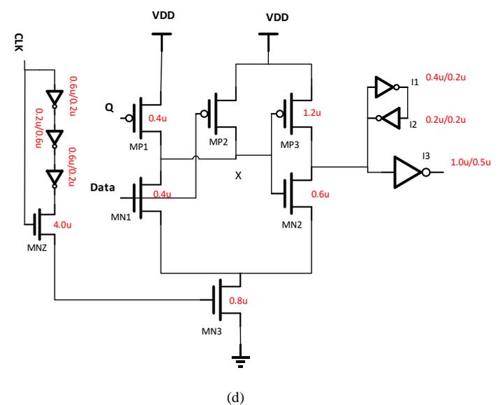
Fig. 2. Conventional P-FF designs: (a) ep-DCO [9] (b) CDFP [12] (c) Static CDFP [19] (d) MHLFF [20]
