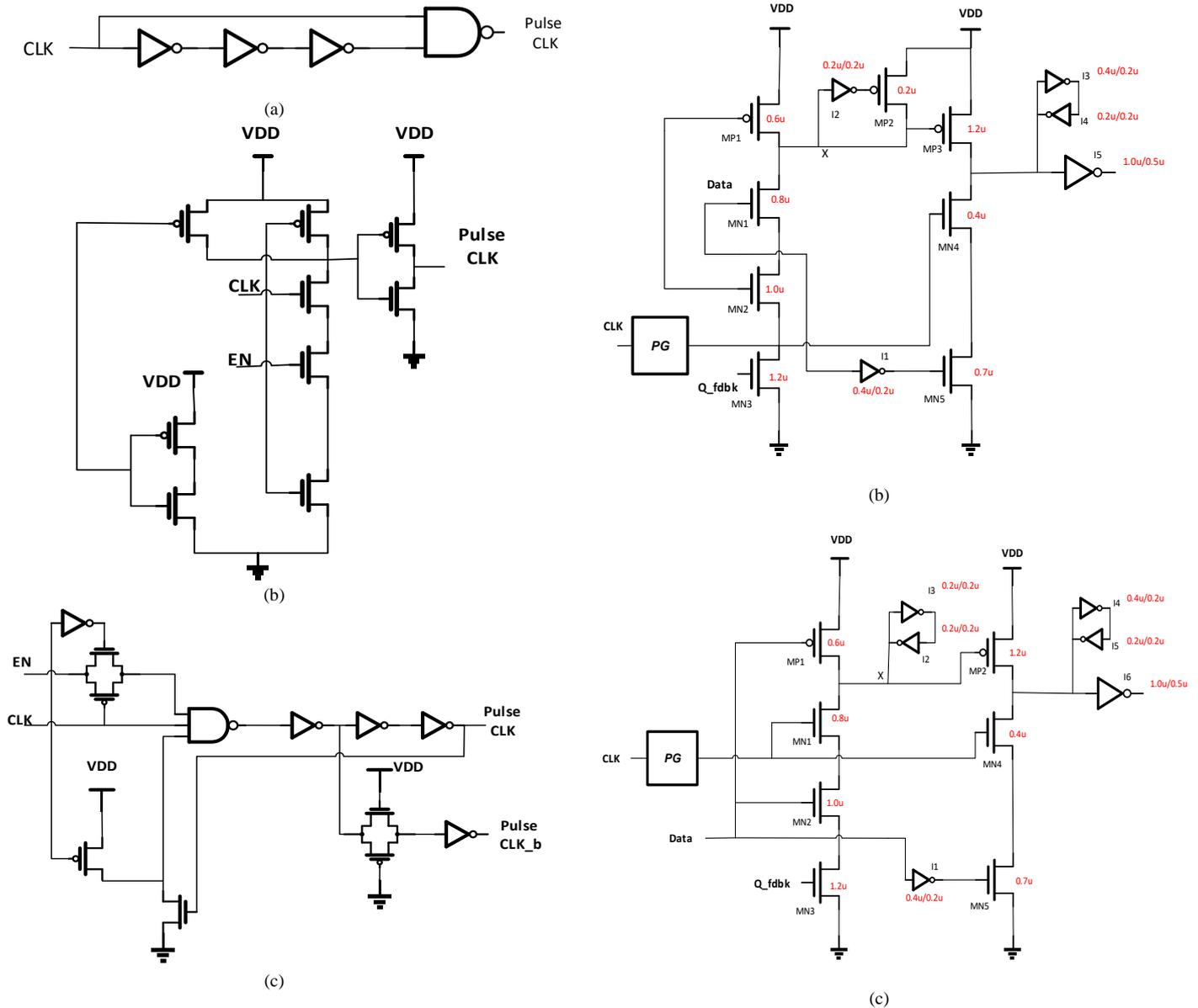
Fig. 1. Pulse generator circuits (a) clock chopper [16] (b) Naffziger [8] (c) NEC RISC processor [17]
