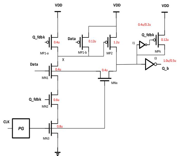
Fig. 5. Modified P-FF based on signal feed-through scheme
