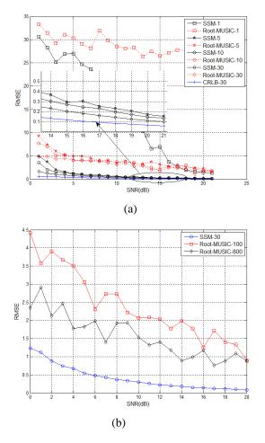
Fig.1.The RMSE of the DOA versus SNR
