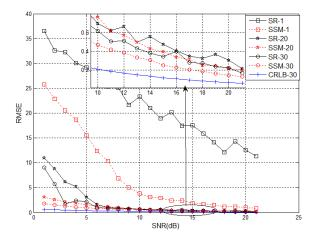
Fig. 7. The RMSE of the DOA versus SNR
