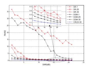
Fig. 2.The RMSE of the DOA versus SNR
