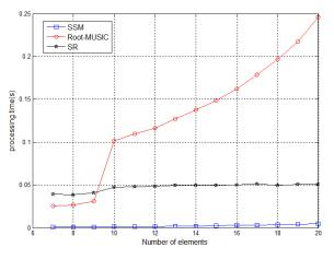
Fig.8. The processing time versus the number of elements
