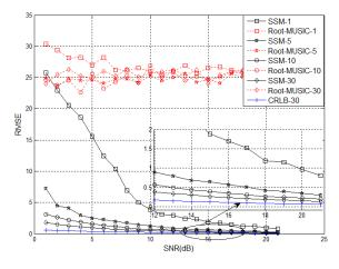
Fig.5. The RMSE of the DOA versus SNR
