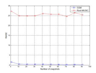
Fig.6. The RMSE of the DOA versus the number of snapshots
