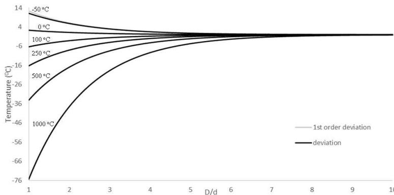
Fig. 2. The deviation of the temperature value due to SSE as a function of the  $D/d$  ratio, calculated from (4) for direct reading RTs and from (8) (the first order approximation) for RTs with the electrical output signal.
