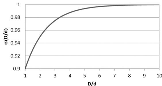
Fig. 1. Expression of the proposed SSE as a function of the source diameter/ field of view ratio, (1).
