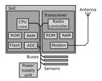
Fig. 3.1. A typical architecture of wireless sensor node.
