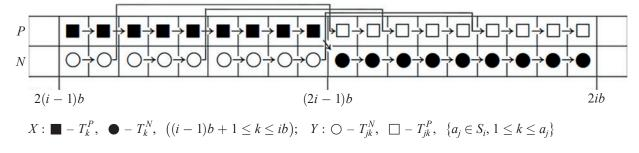
Fig. 4. An example slot of the constructed schedule for P(1), N(1)| chain,  $p_i = 1|C_{max}$
