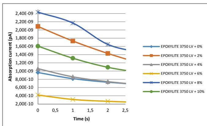
Fig. 8. Absorption currents on samples filled by  $\text{Al}_2\text{O}_3$
