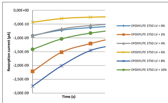
Fig. 9. Resorption currents on samples filled by  $\text{Al}_2\text{O}_3$
