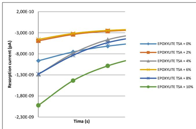
Fig. 11. Resorption currents on samples filled with Al<sub>2</sub>O<sub>3</sub>
