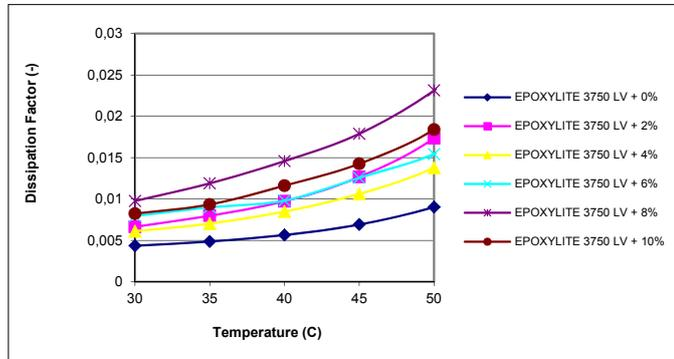
Fig. 3. Measurement of  $\tan\delta$  versus temperature from 30°C to 50°C
