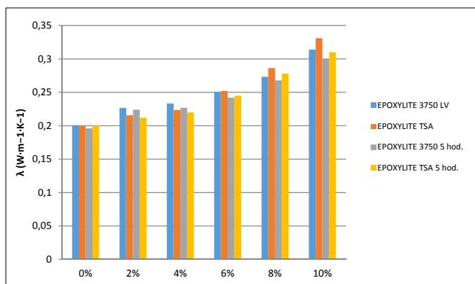
Fig. 1. Thermal conductivity of the samples filled  $\text{Al}_2\text{O}_3$
