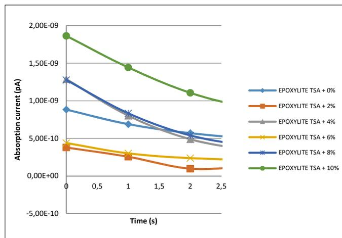
Fig. 10. Absorption currents on samples filled with  $\text{Al}_2\text{O}_3$
