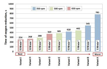
Fig. 6. Quantitative evaluation of the efficiency of each variant according to the time of oxygen content reduction in the water to a value close to 0 ppm
