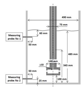
Fig. 3. Basic physical model dimension data
