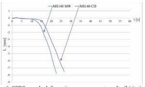
Fig. 6. SSBS sample deformation measurement results (L) in time function, for MS140 (SiO<sub>2</sub>/Na<sub>2</sub>O=3.0): microwave hardened (MW) or classically dried (CD)
