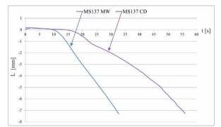
Fig. 5. SSBS sample deformation measurement results (L) in time function, for MS137 (SiO<sub>2</sub>/Na<sub>2</sub>O=3.4): microwave hardened (MW) or classically dried (CD)
