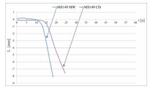
Fig. 7. SSBS sample deformation measurement results (L) in time function, for MS149 (SiO<sub>2</sub>/Na<sub>2</sub>O=2.9): microwave hardened (MW) or classically dried (CD)
