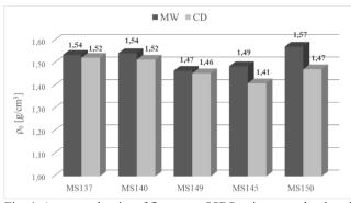
Fig. 4. Apparent density of five types SSBS: microwave hardened (MW) or classically dried (CD)
