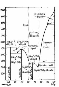
Fig. 3. Two-component system Na<sub>2</sub>O–SiO<sub>2</sub> with marked ranges for commercial sodium silicates [19, 20]
