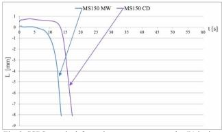
Fig. 9. SSBS sample deformation measurement results (L) in time function, for MS150 (SiO<sub>2</sub>/Na<sub>2</sub>O=2.0): microwave hardened (MW) or classically dried (CD)
