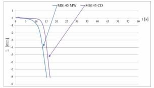
Fig. 8. SSBS sample deformation measurement results (L) in time function, for MS145 (SiO<sub>2</sub>/Na<sub>2</sub>O=2.5): microwave hardened (MW) or classically dried (CD)
