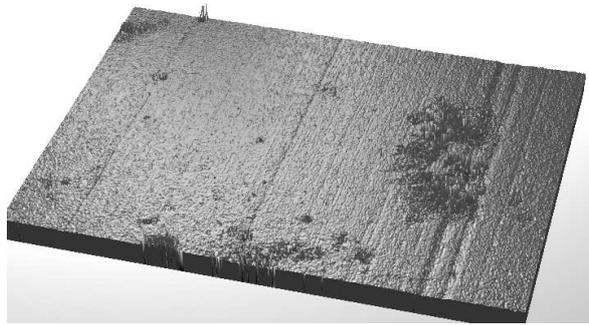
Fig. 6. Brake drum after vitrification, 80 thousands of kilometres of covered distance.
