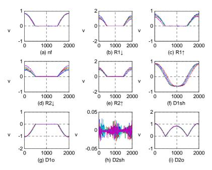
Fig. 12. Waveforms of fault classes for the actual circuit.
