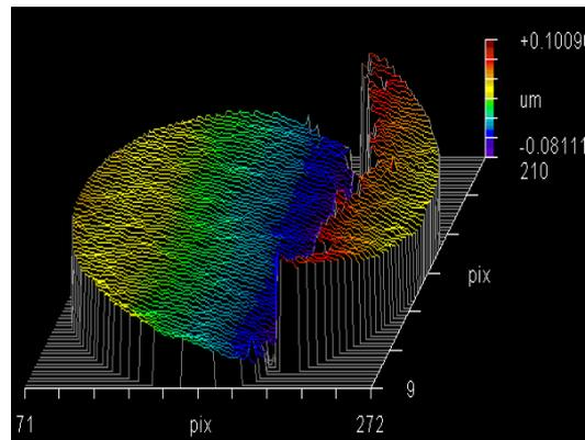
Fig. 3. Analysis of surface flatness by laser interferometer.
