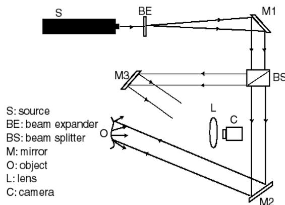
Fig. 1. The scheme of the holographic technique.
