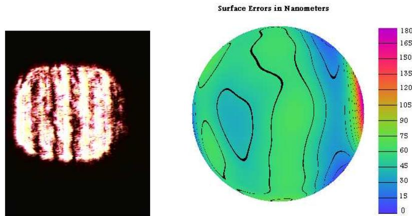
Fig. 2. Analysis of surface flatness using digital holography.
