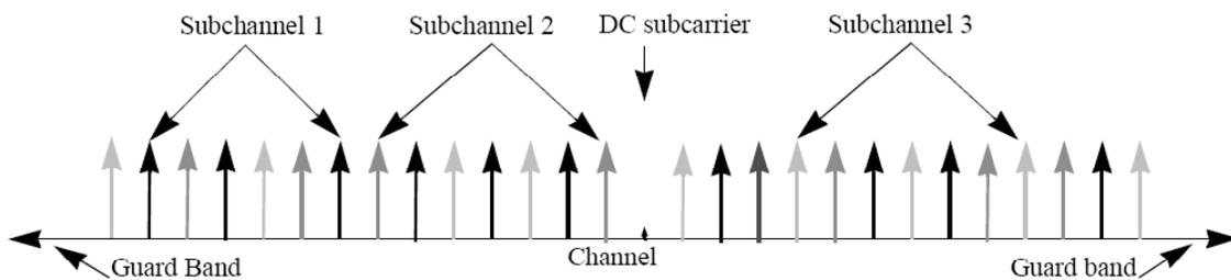
Fig. 1. Example of channel subdivision for standard 802.16d using the OFDMA mode.
