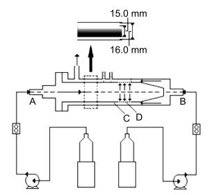
Fig. 3. Scheme of tube-in-tube microchannel reactor. A-inlet of inner tube; B-inlet of outer tube; C-microchannel; D-micropores. Adapted from (Yang et al., 2010) with permission from American Chemical Society (Copyright, 2010)
