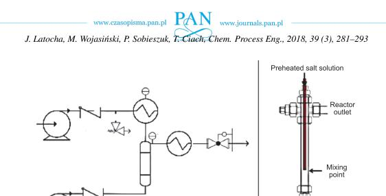
Fig. 2. Scheme of continuous hydrothermal synthesis (left) and hydrothermal rig (right). Reprinted from (Lester et al., 2012) with permission from Elsevier (Copyright, 2011)
