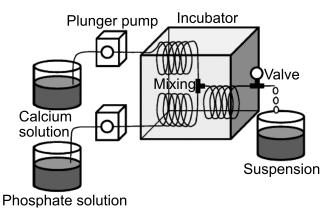
Fig. 1. Production of hydroxyapatite in tube reactor. Reprinted from (Fujii et al., 2015) with permission from The Ceramic Society of Japan (Copyright, 2015)
