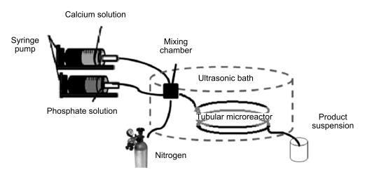
Fig. 5. Scheme of production HAp in ultrasonic tubular reactor. Reprinted from (Castro et al., 2013a) with permission from Elsevier (Copyright 2013)
