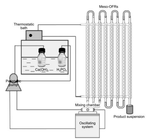
Fig. 6. Scheme of HAp production in scaled-up meso-OFR. Adapted from (Castro et al., 2013b) with permission from American Chemical Society (Copyright, 2013)
