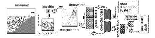
Fig. 1. Sampling points in the water treatment line in the studied heat and power station (detailed description of sites in Material and methods section)
