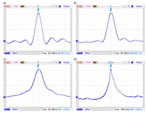
Fig. 4. The behaviour of functions of CAV: the low-pass white noise: N(0 V, 0,3 V), B = 25 kHz and after the noise passed the first-order inertial system with various time constants  $T_c$  (a):  $T_c = 10$  µs (b);  $T_c = 30$  µs (c);  $T_c = 100$  µs (d).
