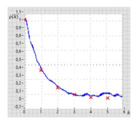
Fig. 5. The experimental behaviour of normalized autocorrelation function  $\rho_x(k\Delta t)$  of the low-pass white noise N(0 V, 0.3 V), B = 25 kHz after it passed the first-order inertial system with a time constant  $T_c = 100 \,\mu s$  (continuous line) and the calculated autocorrelation values (points x).
