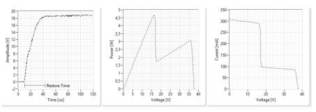
Fig. 10. The response to a short load pulse: voltage (left), power(middle), current – according to the measured I–V curve for partial shading conditions (right).
