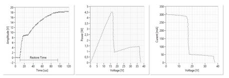
Fig. 11. The response to a short load pulse: voltage (left), power(middle), current – according to the measured I–V curve for partial shading conditions (right).
