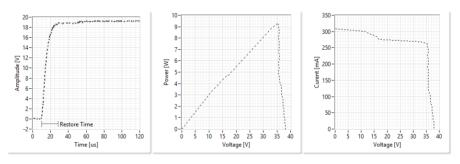
Fig. 8. The response to a short load pulse: voltage (left), power(middle), current – according to the measured I–V curve for partial shading conditions (right).
