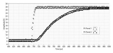
Fig. 3. The PV Panel 1 response for full insolation and the PV Panel 2 response for partly shaded conditions.
