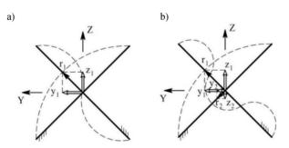
Fig. 7. The effect of a plate waveform on the movement of the device output axis.
