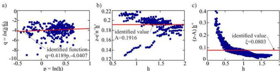
Fig. 5. Visualization of determining the hysteresis parameters: identification of  $\nu$  and  $n$  values using the least square method (a); identification of  $A$  value (b); identification of  $\zeta$  value (c).
