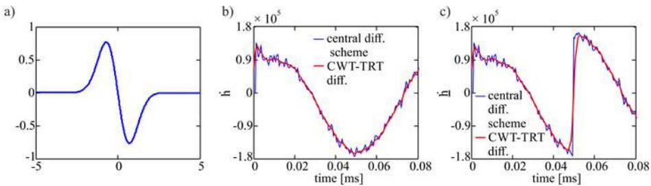
Fig. 4. Noise reduction for the hysteresis derivative: Gaussian wavelet of order 1 (a); comparison of finite difference and CWT-TRT differentiation of  $\dot{h}$  (b); comparison of finite difference and CWT-TRT differentiation of  $\dot{\underline{h}}$  (c).
