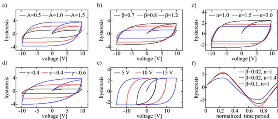
Fig. 1. Variability of the hysteresis component according to (2) for the following parameters:  $\beta = 0.8, \gamma = -0.4, n = 1$ (a);  $A = 1, \gamma = -0.4, n = 1$  (b);  $A = 1, \beta = 0.8, \gamma = -0.4$  (c);  $A = 1, \beta = 0.8, n = 1$  (d);  $A = 1, \beta = 0.8, \gamma = -0.4, n = 1$  (e);  $A = 0.5, \gamma = -0.04$  (f).
