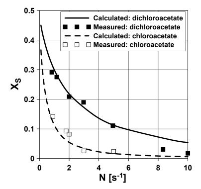
Fig. 7. Effect of agitation rate on selectivity  $X_S$  for ethyl chloroacetate and ethyl dichloroacetate;  $c_B=1M$ ,  $c_{A0}=c_{C0}=0.02M$ ,  $\alpha=50$ , feeding position A close to the impeller
