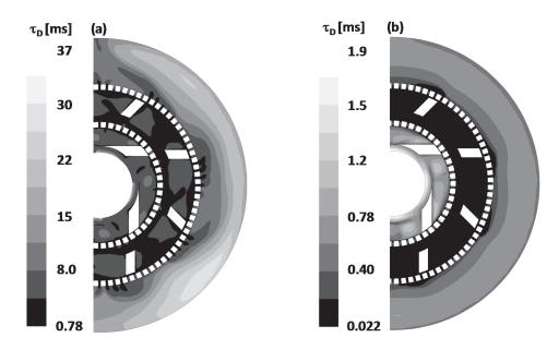
Fig. 12. The time constant for mass transfer of benzoic acid from toluene drops to aqueous solution emulsion for  $\varphi = 0.75 \ \eta_c = 0.91 \text{ mPas}$ ,  $\eta_d = 0.587 \text{ mPas}$ ,  $Q_m = 600 \text{ kg/h}$  (a) N = 1000 rpm, (b) N = 11000 rpm
