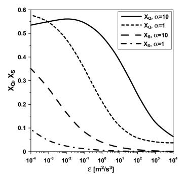
Fig. 8. Predicted effect of the energy dissipation rate,  $\varepsilon$ , on product distributions  $X_Q$  and  $X_S$ : for  $\alpha = Q_A/Q_B = 1$ ,  $c_{A1,0} = 1.2 \text{ mol/m}^3$ ,  $c_{A2,0} = 2.4 \text{ mol/m}^3$ ,  $c_{B0} = 1 \text{ mol/m}^3$ , for  $\alpha = Q_A/Q_B = 10$ ,  $c_{A1,0} = 1.2 \text{ mol/m}^3$ ,  $c_{A2,0} = 2.4 \text{ mol/m}^3$ ,  $c_{B0} = 10 \text{ mol/m}^3$
