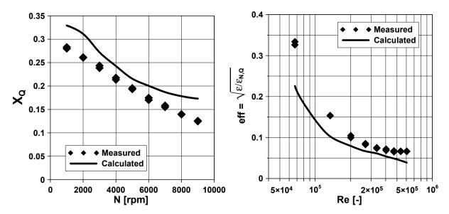
Fig. 10. Dependences of the product distribution  $X_Q$  on the rotor speed and efficiency of mixing *eff* on the Reynolds number, Re
