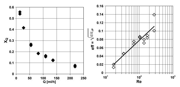
Fig. 11. Dependences of the measured product distribution  $X_Q$  on the flow rate and efficiency of mixing eff on the Reynolds number, *Re* (based on Malecha et al., 2009)
