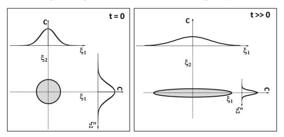
Fig. 1. Effect of stretching on spreading of the contaminant due to molecular diffusion
