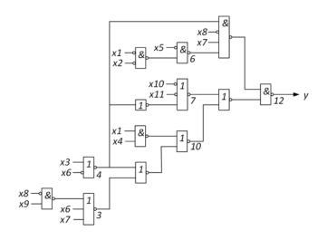
Fig. 10. Example 2 with NOR and NAND gates.
