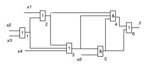
Fig. 11. Example 3 with OR and AND gates.
