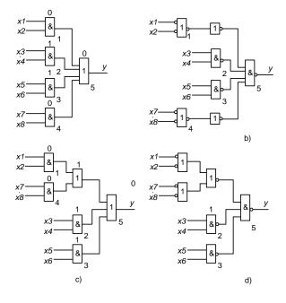
Fig. 14. Splitting of a gate in NOR-NAND circuit.
