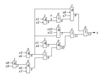
Fig. 9. Example 2 with AND and OR gates (marked).
