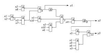
Fig. 5. Final step of the mapping with NAND gates.
