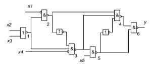
Fig. 13. Example 3 with NOR and NAND gates.
