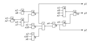
Fig. 8. Example 1 with NOR and NAND gates.
