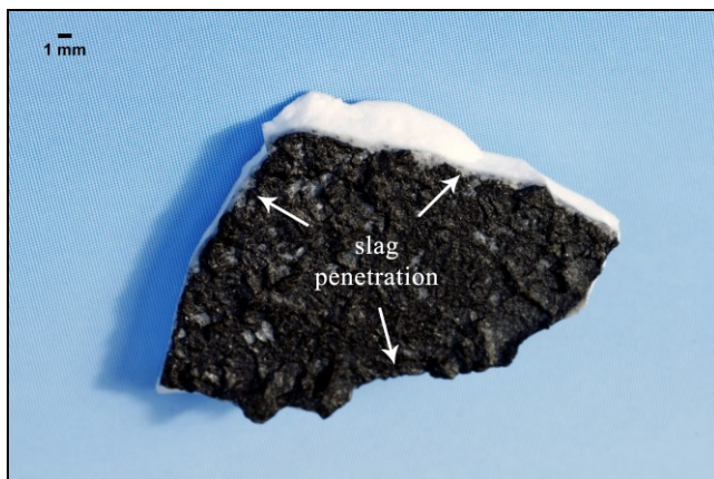
Fig. 5. View from the top of the corundum crucible after the measurement of slurry slag at 1360°C (natural size)
