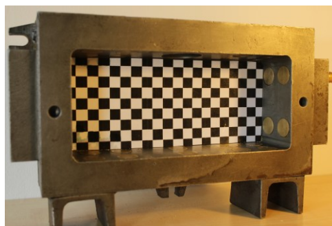
Fig. 2. Core box R-1 version, nominal cavity volume: 808.4 cm 3
