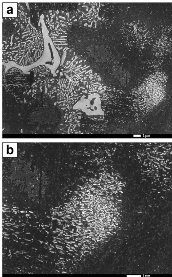
Fig. 7. SEM image of discontinuous and continuous precipitates near the eutectic region (a); high magnification (b) revealing locally observed continuous precipitates. Alloy solidified in a mould with an initial temperature of 20 °C
