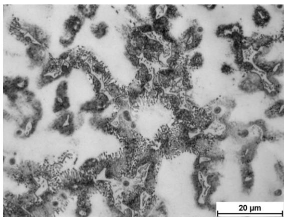
Fig. 6. Microstructure of AZ91 alloy in the T5 temper; alloy solidified in a mould with an initial temperature of 20 °C
