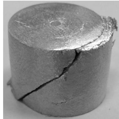
Fig. 5. AZ91 alloy sample after the compression test
