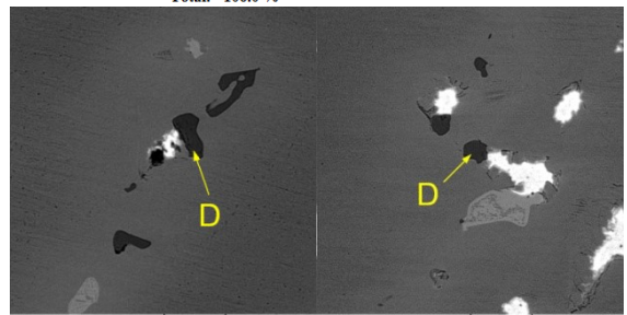
Fig. 9. EDS of the intermetallic compound of iron-nickel-phosphorus (particle D)
