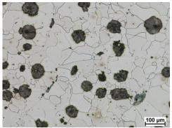
Fig. 3. Ductile cast iron, magnification 100x
