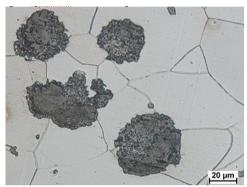
Fig. 4. Ductile cast iron, magnification 500x
