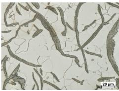
Fig. 6. Grey cast iron, magnification 500x
