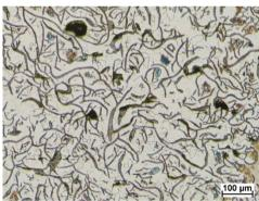
Fig. 5. Grey cast iron, magnification 100x
