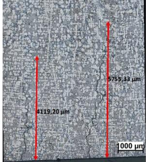
Fig. 8.Macroscopic view of samples after cycles of test and view of microstructure with marked length of cracks- Ductile cast iron
