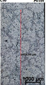
Fig. 9.Macroscopic view of samples after cycles of test and view of microstructure with marked length of cracks- Grey cast iron
