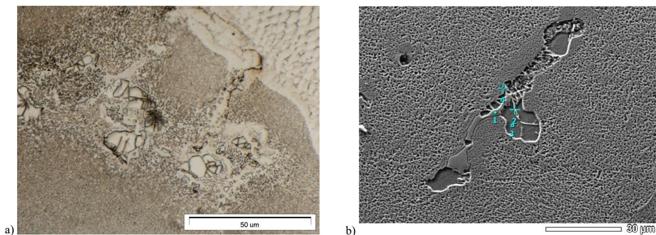
Fig. 5. The microstructure of the IN 713C with the ( $\gamma + \gamma'$ ) eutectic islands: a) LM, b) SEM
