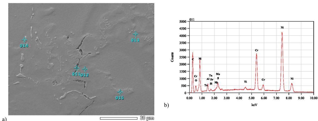
Fig. 6. a) The crack identified in the structure of the pad weld, b) The chemical composition of the crack
