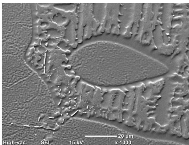
Fig. 4. The fusion line with the PFZ area
