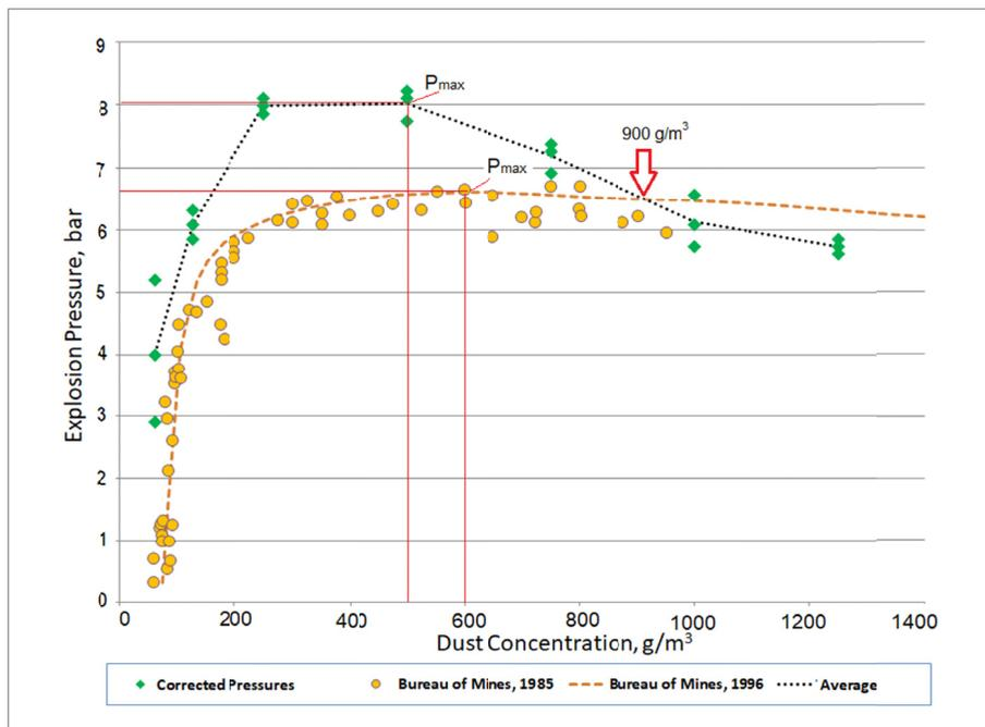
Fig. 6. Explosion Pressure – MS&amp;T Data with Referenced Data (Cashdollar et al., 1985; Cashdollar, 1996)
