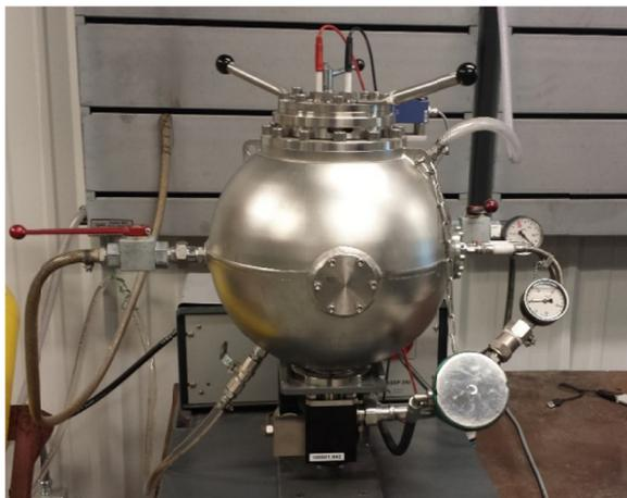
Fig. 4. Siwek 20-Liter Sphere used for testing
