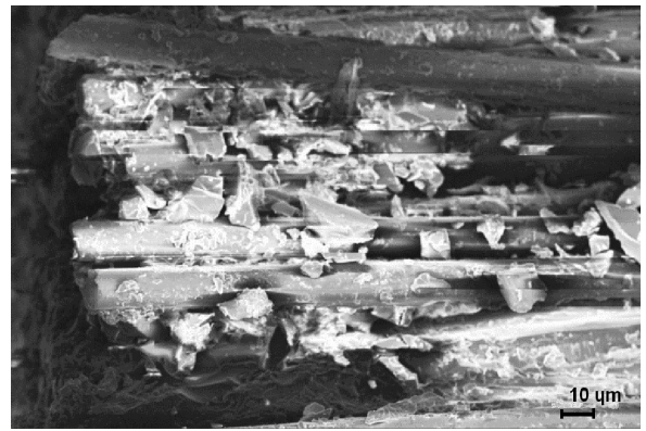
Fig. 7. “Mishmash” structure clearly visible on the side surface of the aged sample, magnified 500 times
