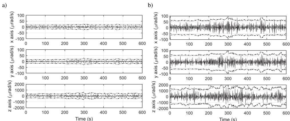
Fig. 4. The angular velocity estimate error and  $3\sigma$  boundary. New method (a); M2 method (b).
