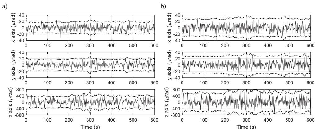
Fig. 5. The attitude estimate error and  $3\sigma$  boundary. New method (a); M2 method (b).
