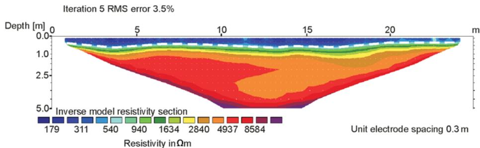
Fig. 2. The results of the shallow ERT surveys profiling on the Storflaket mire near Stordalen. The white broken line shows the depth of the active layer.
