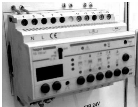
Fig. 1. The Tebis system module TS 100 by Hager
