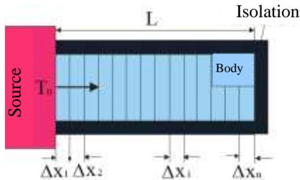
**Fig. 3.** Diagram of heat energy transfer in the rod with the isolated surface
