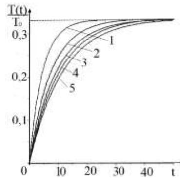
Fig. 7. Aperiodic dynamic characteristics of the heat energy transfer process
