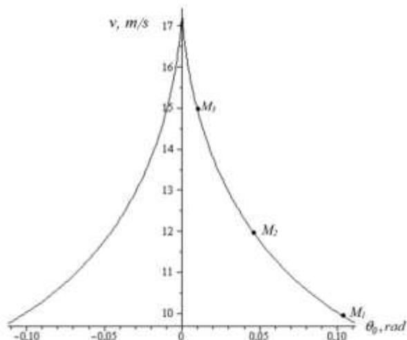
**Fig. 2.** Critical set of longitudinal velocity control parameters  $v$  and the rotation angle of the controlled wheel module ( $k = 400$  H·m)
