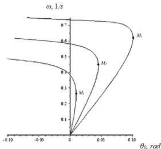
**Fig. 3.** Equilibrium curves of the corresponding angular speeds  $\omega$  of the stationary modes at the change of the rotation angle of the controlled wheel module  $\theta_0$ ; ( $k=400$  Nm;  $v=15$ ; 12; 10 m/s)
