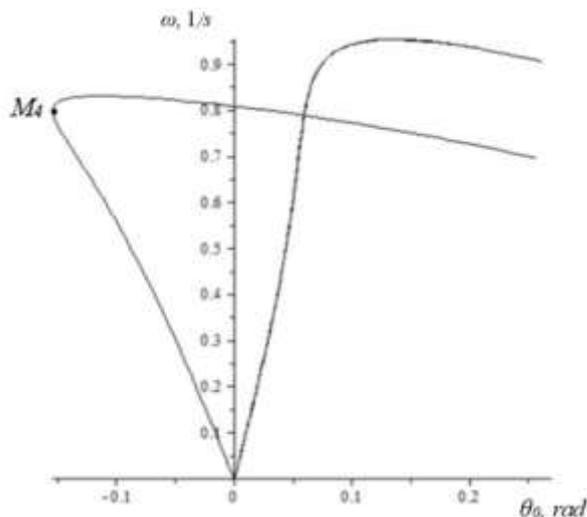
**Fig. 5** Equilibrium curves of the corresponding angular velocities  $\omega$  of stationary modes while changing the pivot point of the controlled wheel module  $\theta_0$ ; ( $k=40$  Nm;  $v=6$ ; 8 m/s)
