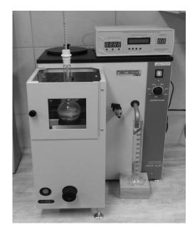
**Fig. 3.** Photo bench equipped with a distiller HAD 620/1 by Herzog
