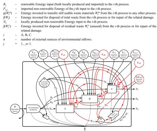
Fig. 2. System diagram of an integrated production system, in which the waste released by one process is at least partially used as raw resource by another process. Circularity paths are highlighted in red.  $P_i$  – mass of product(s) from the *i*-th process
